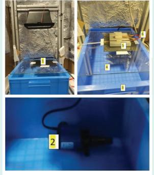
1. Black Paper 2. Pump 3. Tank 4. Glass 5. Aluminium Heat Sink 6. Copper Tube
